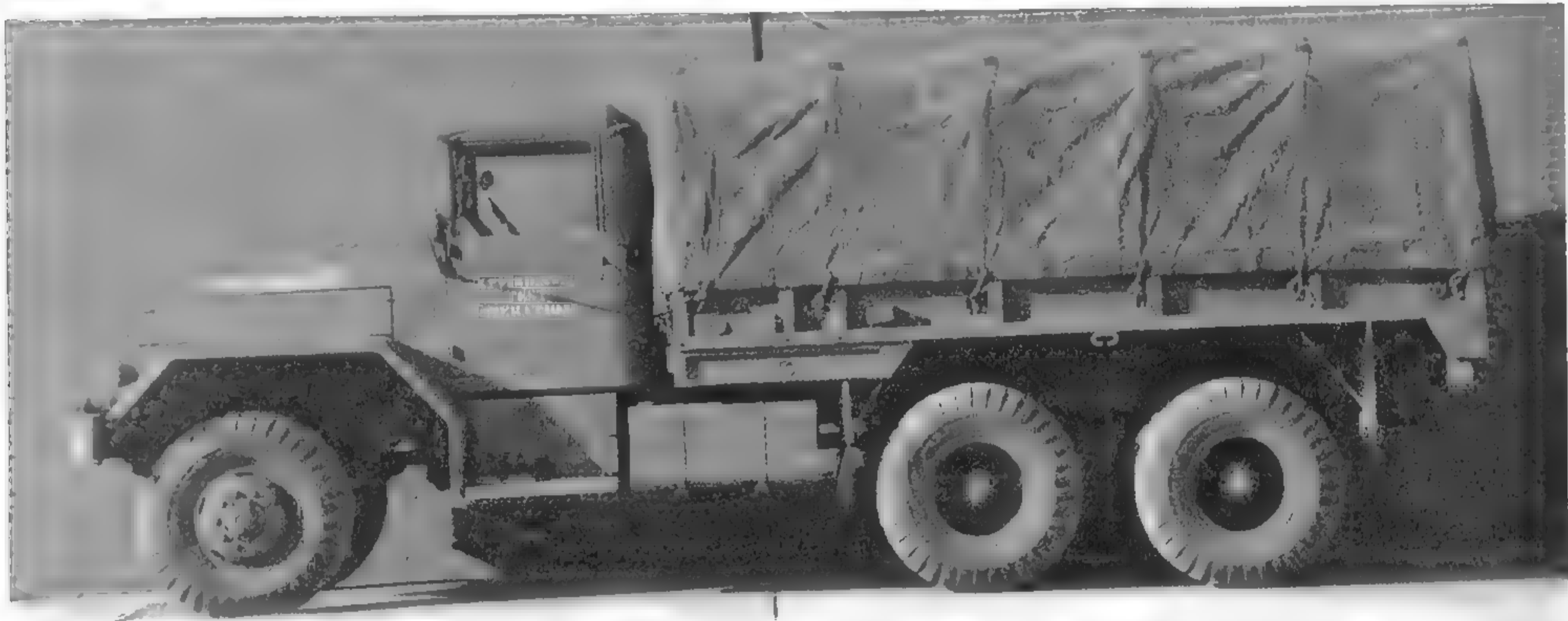
While the shared-cab design of the G-742 and G-744 meant the 5-tons resembled the 2 1/2-ton trucks, the fuel tanks were on opposite sides, aiding identification. (Photo courtesy of the Patton Museum)
